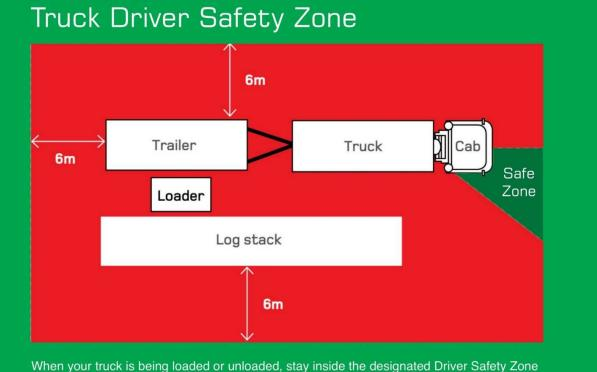
When your truck is being loaded or unloaded, stay inside the designated Driver Safety Zone unless otherwise instructed. Do not stand beside or behind the truck while loading or unloading operations are in progress.
